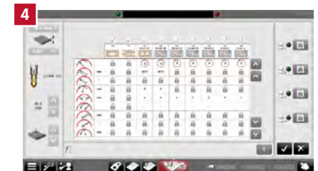
ULTRA SHARP2 function integrated database offering up to 10 cutting qualities
