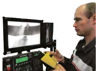
System with large color screen 15", miniaturised camera and additional lighting
